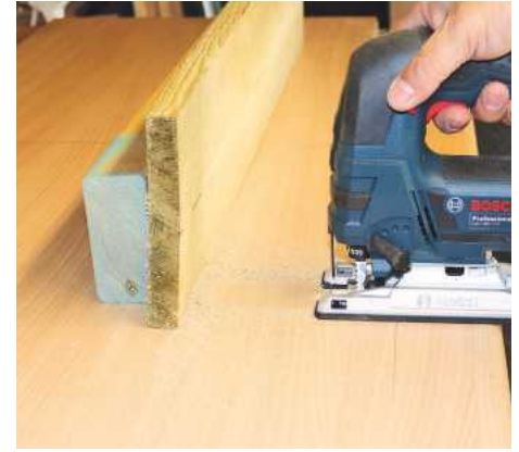
▲ Each saw was also tested for how close it would get to a vertical surface
